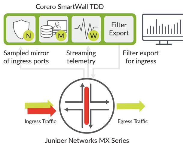
Figure 2: Juniper + Corero DDoS protection joint solution
