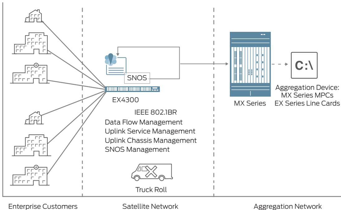
Figure 2. Satellite devices are managed by the MX Series Aggregation device via the IEEE 802.1BR control plane. Satellite device statistics and system logs are all managed by the Aggregation device, greatly streamlining operations.
