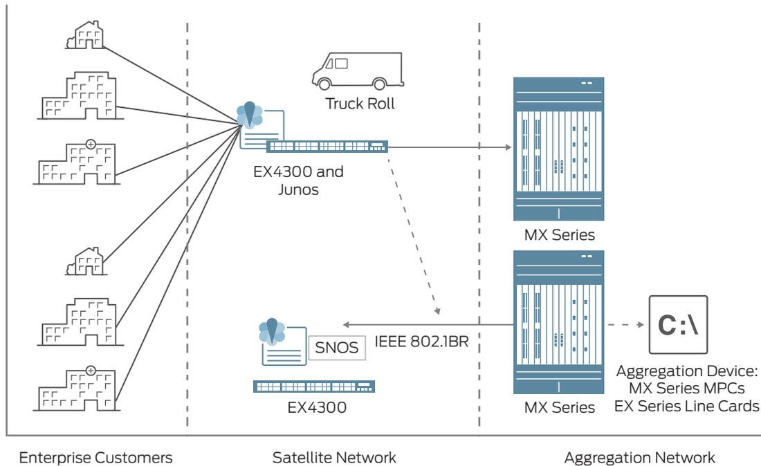
Figure 1. The MX Series Aggregation device automatically discovers and programs Satellite devices with the Satellite Network Operating System (SNOS). Satellite devices appear as extended ports in the router's CLI, along with its native physical line cards.
