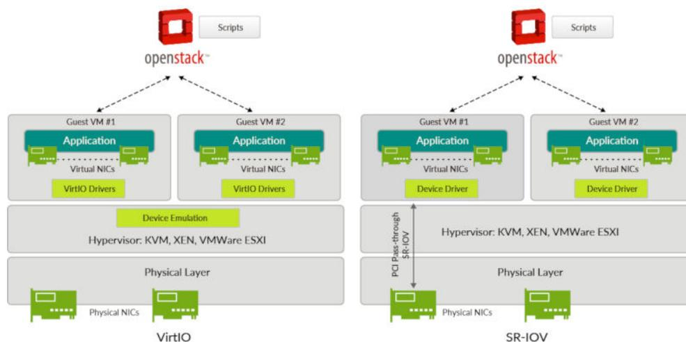
Figure 1: The vMX architecture for VirtIO and SR-IOV.
